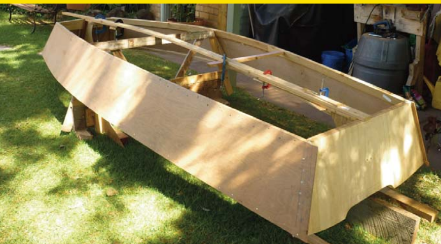
ABOVE: Minimal curves in hull makes construction a lot easier
