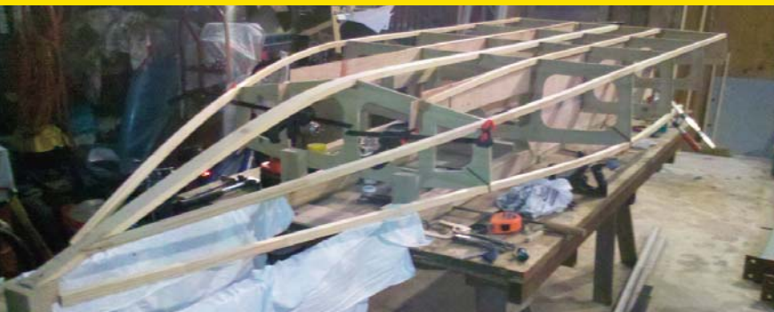
ABOVE: Bulkheads in and ribbing for hull sheeting fitted
