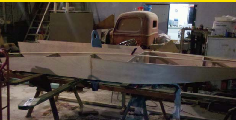
ABOVE: Hull sides and cockpit sides installed.
