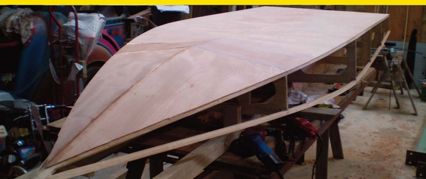
ABOVE: Hull fastened on
