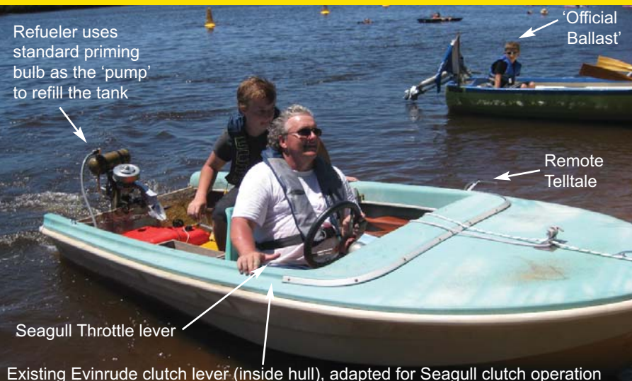
ABOVE: Mark and son Jasper, 16, beaching the 11ft Caribbean 'speed' boat. Note the remote fuel filler, remote telltale and remote throttle (ideas 'borrowed' from the Kiwis) and the custom tiller for steering cables and Clutch cable
