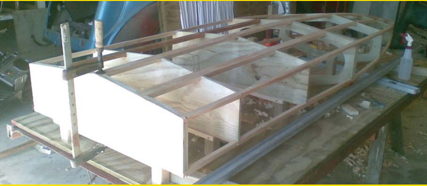
ABOVE: Only the two bow frames have been pre-cut, with the amidships frames left solid to assist with stiffness during construction
