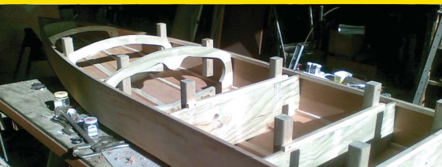
ABOVE: Here, with the deck beams installed, you can clearly see the 3 X 2in temporary 'posts' that kept everything straight whilst upturned
