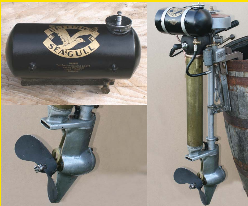
ABOVE: The "after" pics. Authentic gloss black paint on the tank, with repro age-related Seagull logo; cleaned rebuilt and polished gearbox; the completed motor, ready for use if Terry can bear to do so!
