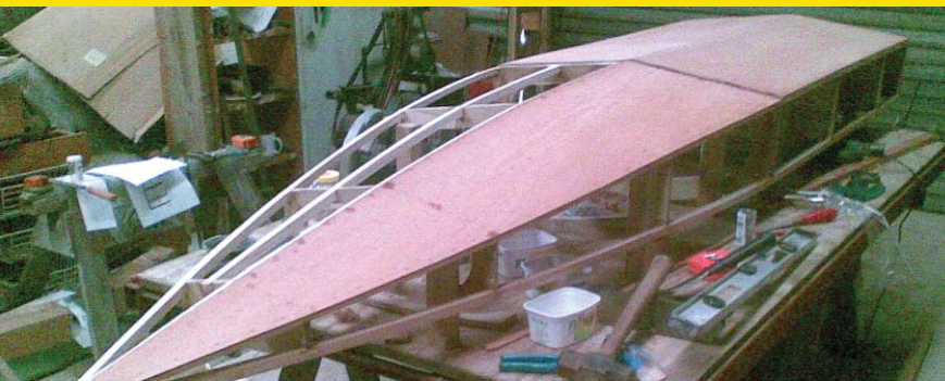
ABOVE: Part way through skinning the hull in 4mm marine ply
