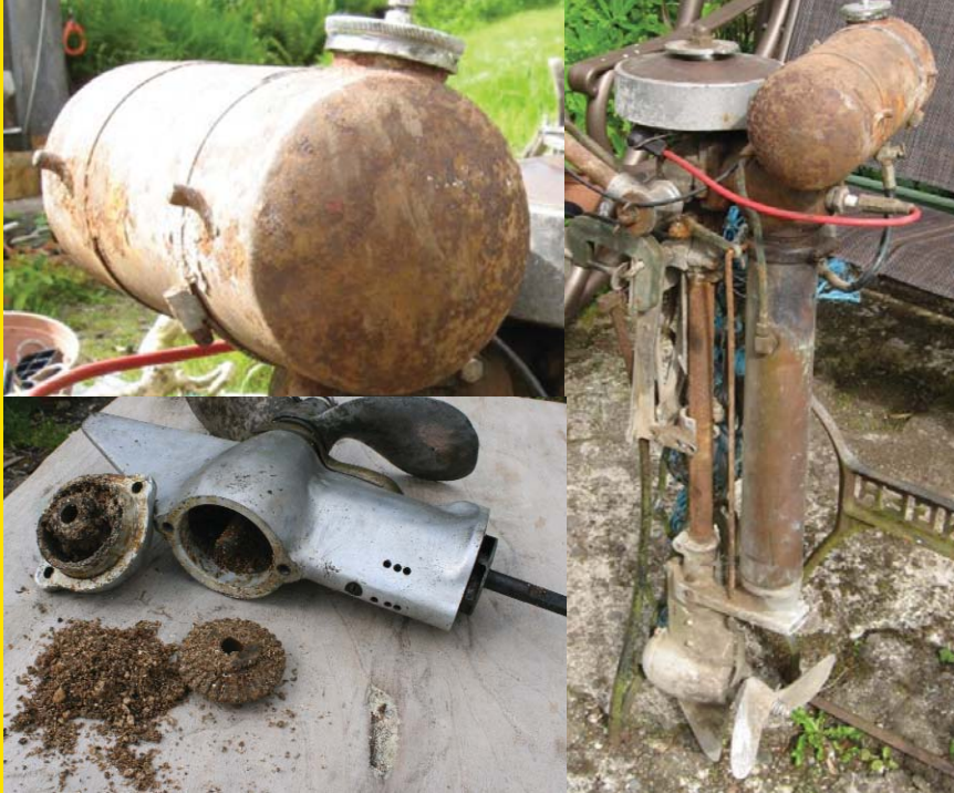
ABOVE: The "before" pics. Rust tank and driveshaft, corrosion everywhere, and look at the muck that came out of the gearbox!
